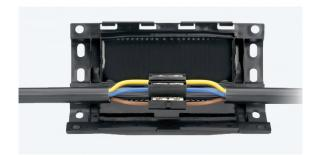
The gel-filled cable joint technique is a new system with special advantages. It is quick and easy to install and reduces the chance of assembly errors. The impact-resistant case is connected by a hinge for easy installation.
